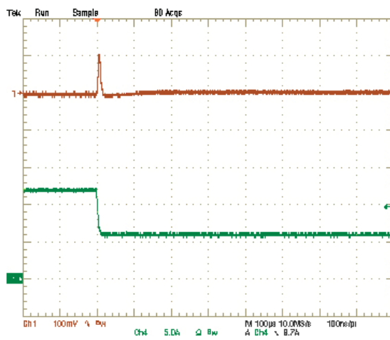
Step Load Transient Response (Vin=5.0V, Vout=3.3V, Cload=94µF, Iout=12A to 6A) Trace 1=Vout, 100 mV/div, Trace 4=Iout, 5A/div.
