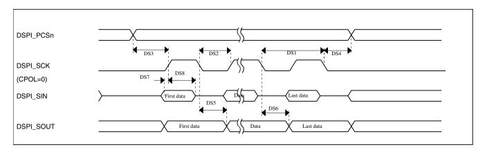
Figure 17. DSPI classic SPI timing — master mode
