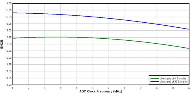
Figure 12. Typical ENOB vs. ADC\_CLK for 16-bit single-ended mode
