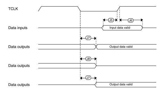
Figure 6. Boundary scan (JTAG) timing
