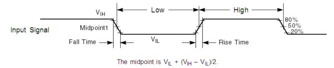
Figure 2. Input signal measurement reference
