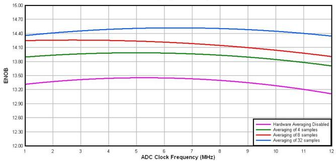
Figure 11. Typical ENOB vs. ADC\_CLK for 16-bit differential mode
