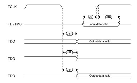
**Figure 7. Test Access Port timing**
