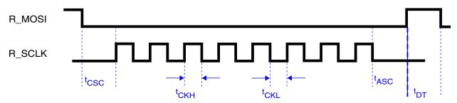
Figure 23. SPI timing: R\_SSEL\_B to R\_SCLK
