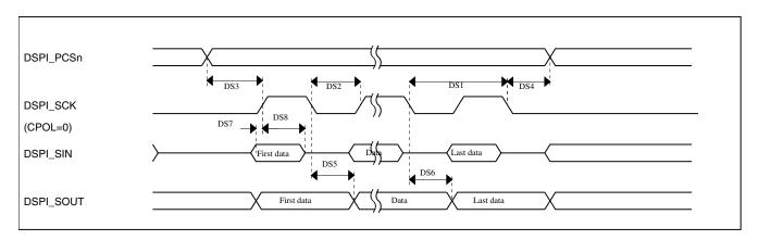
Figure 15. DSPI classic SPI timing — master mode
