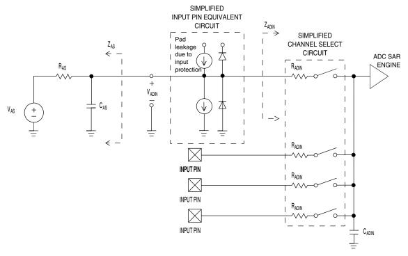
Figure 10. ADC input impedance equivalency diagram
