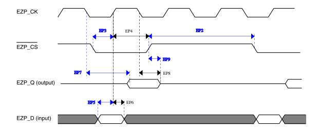
Figure 9. EzPort Timing Diagram
