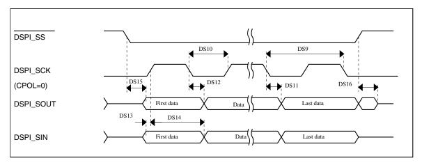
Figure 18. DSPI classic SPI timing — slave mode
