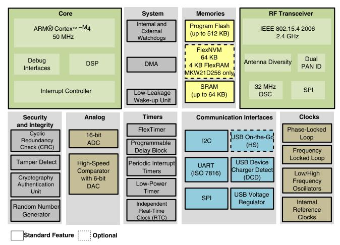
Figure 1. MKW2xDxxxV simplified block diagram
