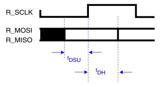
Figure 24. SPI timing: R\_SCLK to R\_MOSI and R\_MISO
