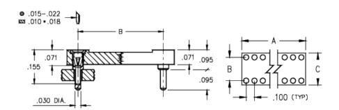
**Description:** DIP Socket Solder Tail Ultra Low Profile (0.095 Tail) Open Frame Through Hole Plating Code: 93 Shell Plating: 200 μ" Tin/Lead(93/7) over 100 μ" Nickel Inner Contact Plating: 30 μ" Gold over 50 μ" Nickel
