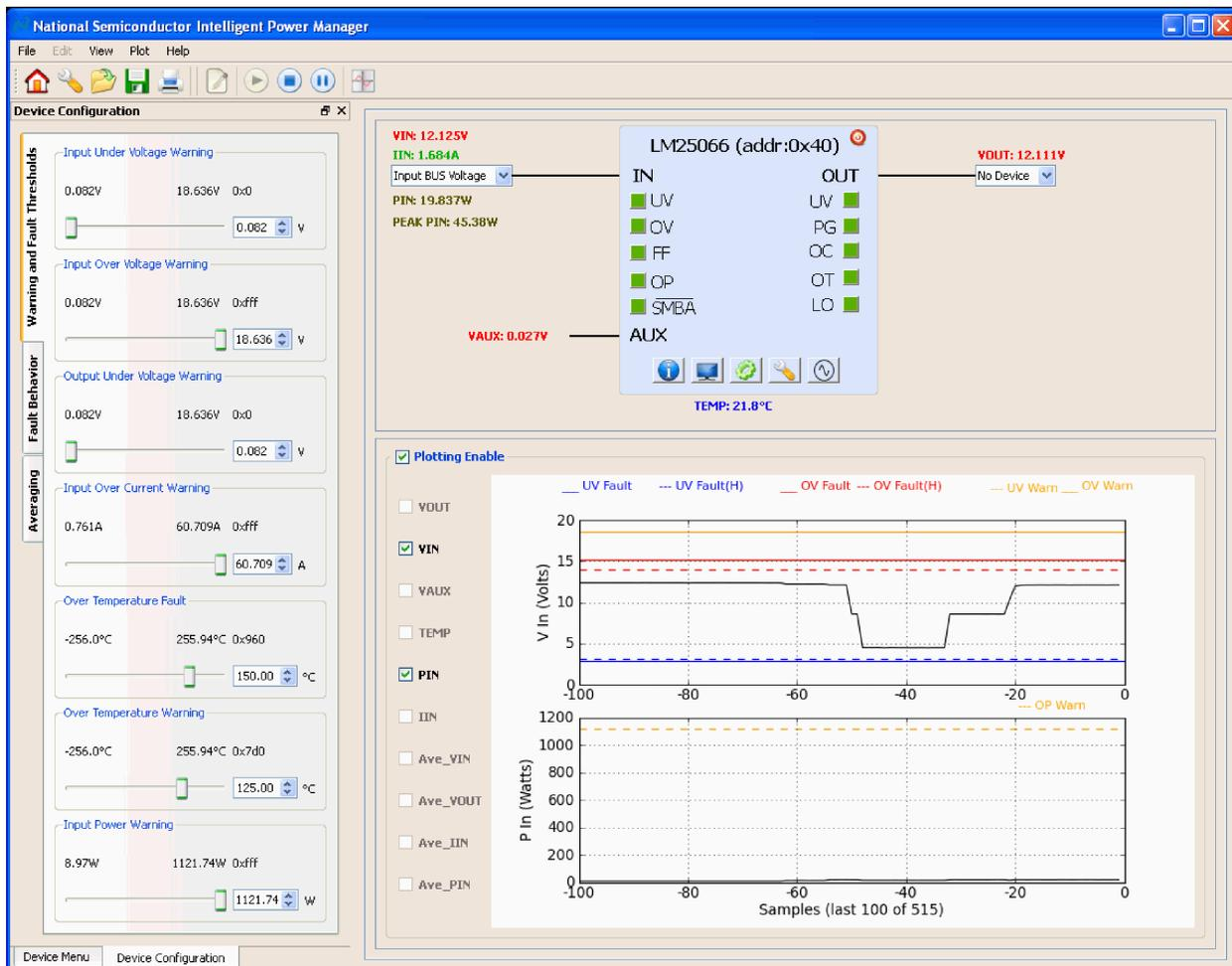
Figure 6. LM25066 GUI with Telemetry Plotting Tool Enabled
