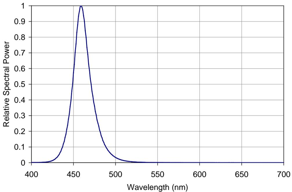
Figure 5: Typical relative spectral power vs. wavelength @ T<sub>c</sub> = 25°C.
