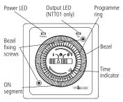
**Time control segments:** 1 segment = 15 minutes, push segment down for ON, pull up for OFF. Control switch:
