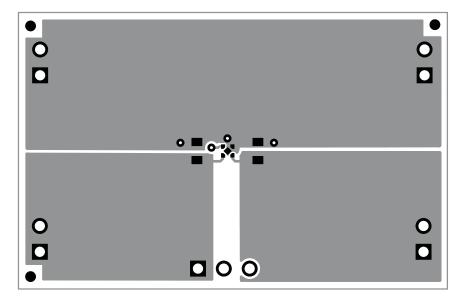
Figure 4. Top Layer Routing
