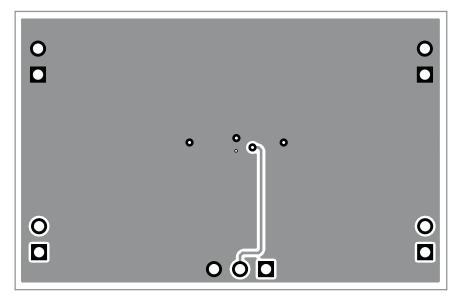
Figure 5. Bottom Layer Routing
