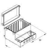
SPECIFICATION Materials Box: Polycarbonate ABS UL94-V0 Lid: Polycarbonate UL94-V0 Heat resistant up to 120°C Operating Temperature Ingress protection class IP65 Light grey, similar to RAL 7038, Transparent lid Standard colours Standard unit includes Box, lid, hinges, catch, fixing screws and neoprene gasket
