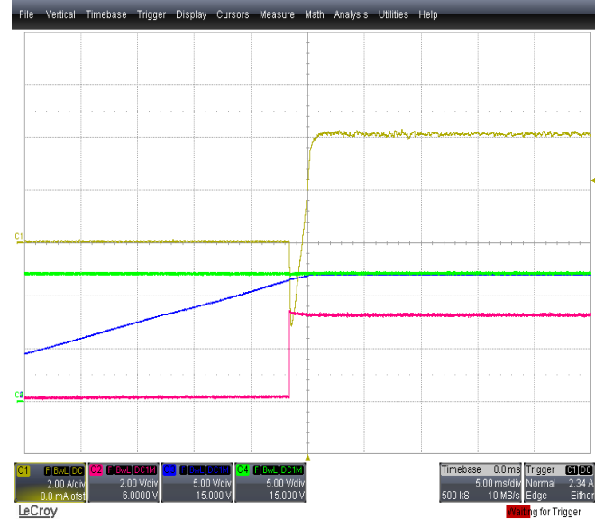
Figure 59 – Output reverse current protection, OrFET enable threshold -384mV Red trace: OrFET gate signal Green and Blue trace: Output voltages of two power supplies Yellow trace: Load current of power supply that is softstarting
