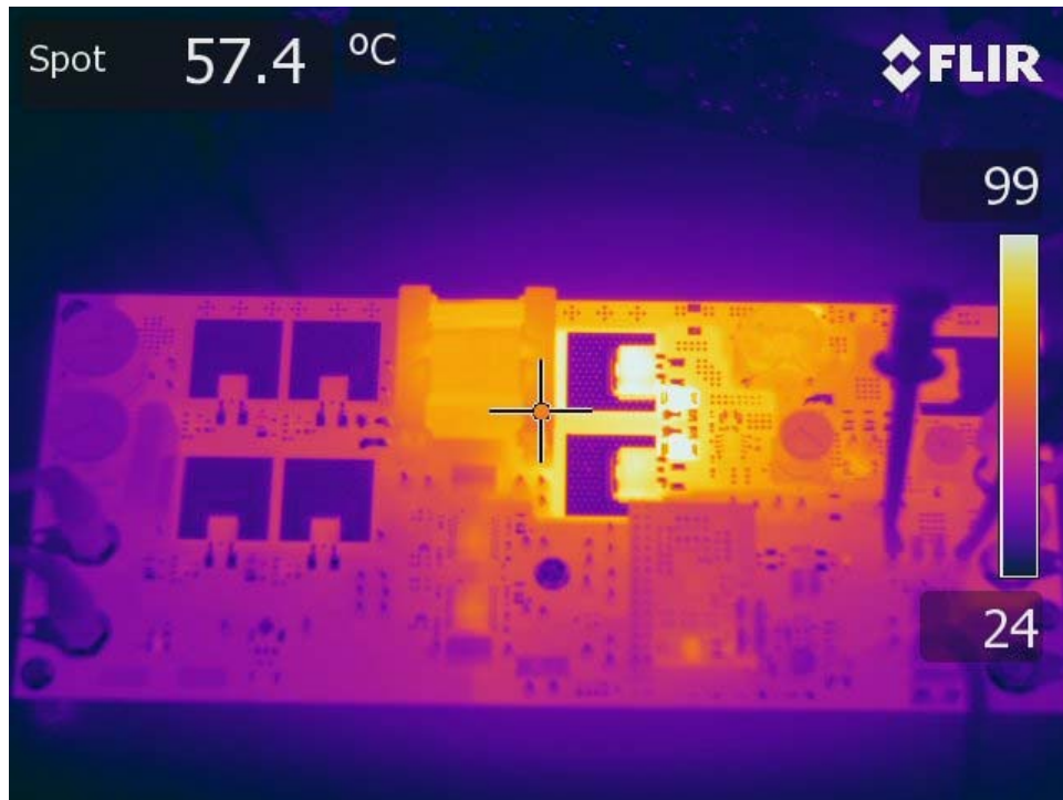
Figure 94 – Thermal image at 60 VDC, 8A load, no air flow, 1 hour soaking time.
