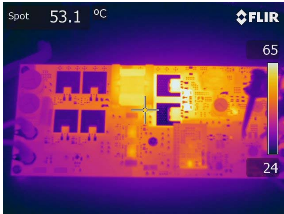
Figure 92 – Thermal image at 36 VDC, 8A load, no air flow, 1 hour soaking time.
