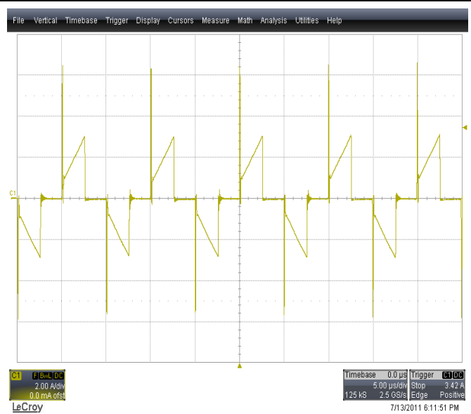
Figure 26 - Primary current after Volt Second Balance implemented, 8A load
