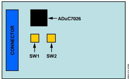
Figure 9. ISEB Switch Locations for Flashing the Microcontroller
