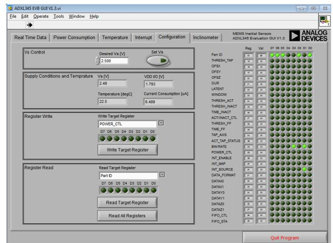
Figure 23. Configuration Tab
