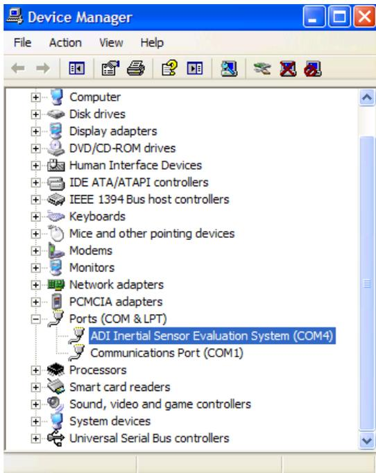
Figure 6. Device Manager Showing the COM Port Number
