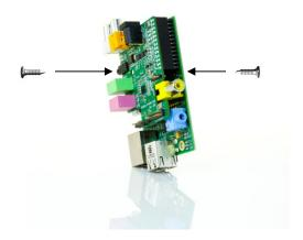
Diagram 3: The Audio Card must be secured to Raspberry Pi with the supplied pillar and screw set.
