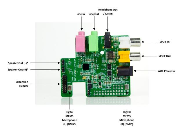
Diagram 1: Connections to and from the Wolfson Audio Card
