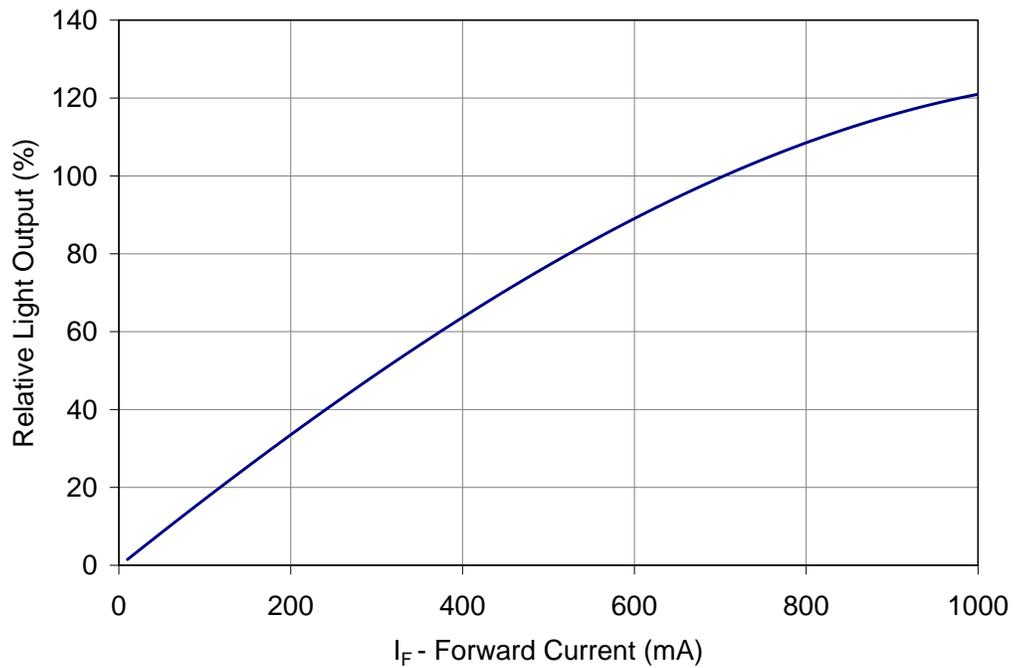
Figure 7: Typical relative light output vs. forward current @ T<sub>c</sub> = 25°C.
