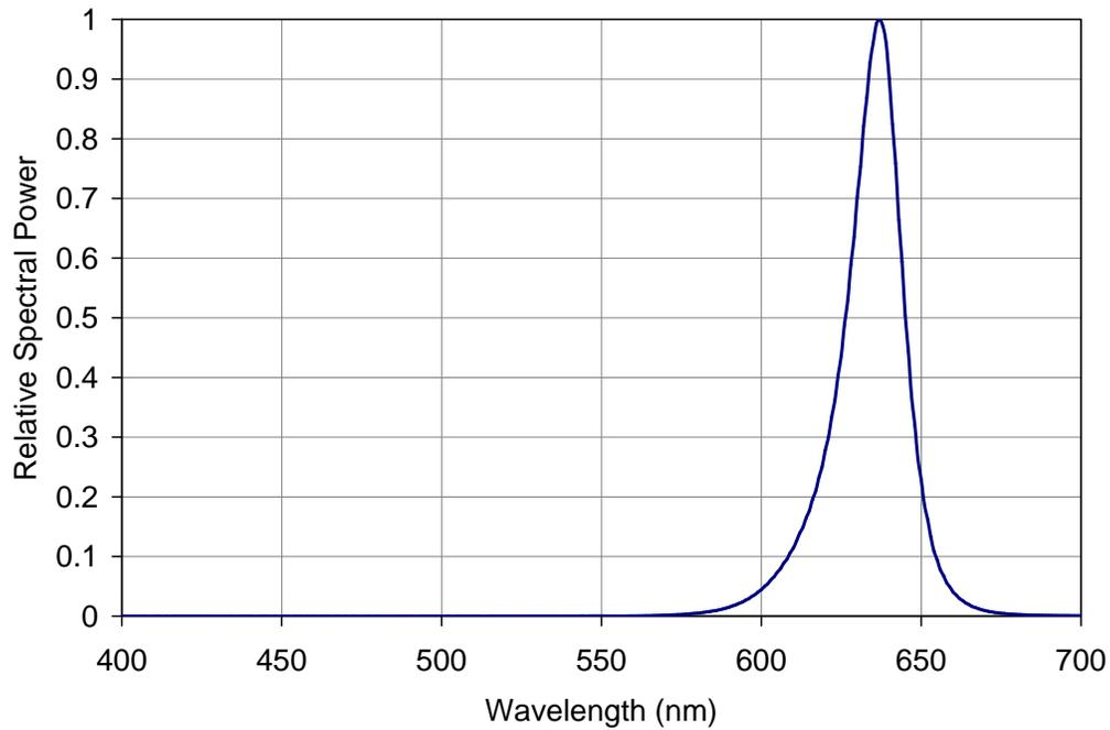
Figure 5: Relative spectral power vs. wavelength @ T<sub>c</sub> = 25°C.
