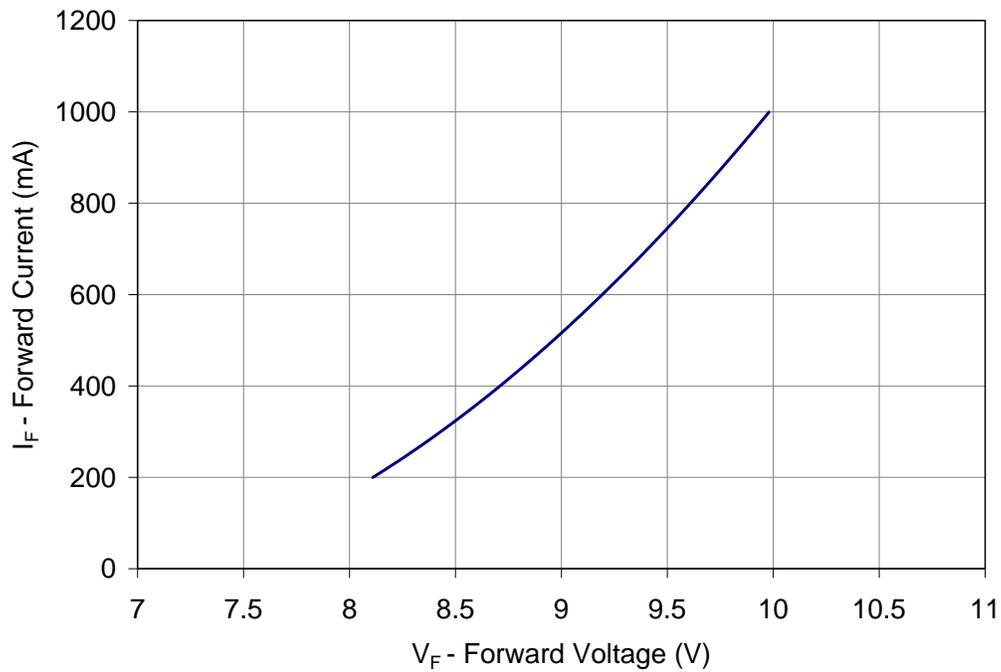
Figure 9: Typical forward current vs. forward voltage @ T<sub>c</sub> = 25°C.
