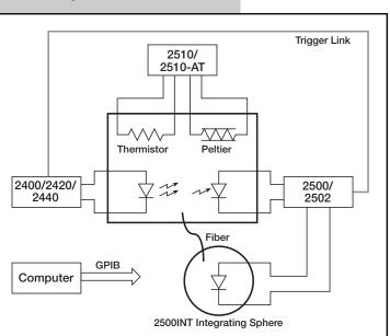
The Model 2500 and Model 2502 are designed for tight integration with other Keithley instruments that are often used in L-I-V test systems for laser diode modules. These other instruments include the Model 2400 SourceMeter and Model 2510 TEC SourceMeter instruments.
