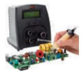
The DX-350 includes an adjustable vacuum-driven "suckback" to control material "tailing" and waste.
