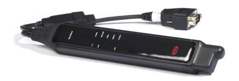
Kvaser BlackBird SemiPro is a powerful and versatile WLAN solution that is able to function over existing wireless infrastructure or to generate it's own 'hotspot' wireless network.
