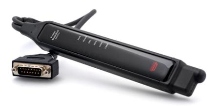
Kvaser BlackBird SemiPro is a powerful and versatile WLAN solution that is able to function over existing wireless infrastructure or to generate it's own 'hotspot' wireless network.
