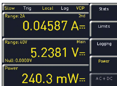
Picture 1: Watt meter in DC range
