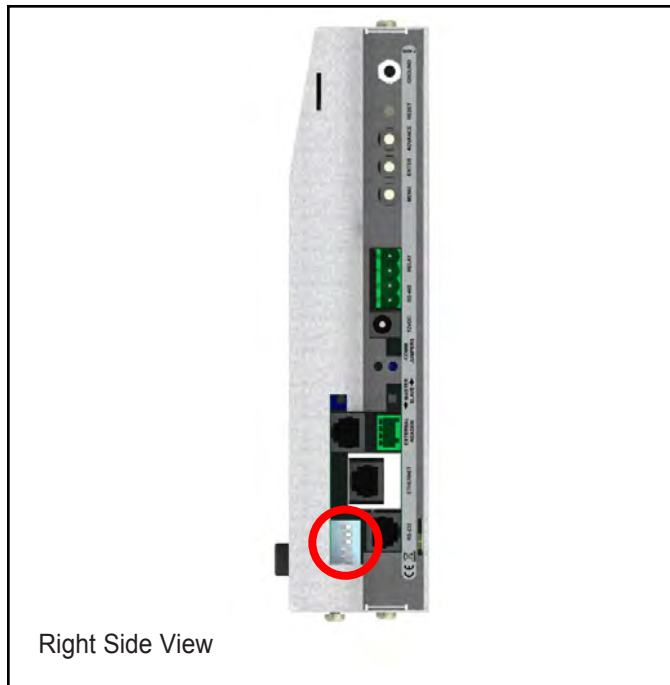
Figure 3. Locating the DIP switch on the SmartLog V5™
