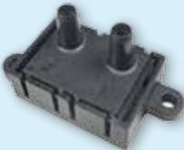
**Airflow sensors:** Advanced microstructure technology. Sensitive and fast response to flow, amount/direction of air or other gas. Analog or digital output. Thin-film, thermally isolated bridge structure consists of a heater and temperature sensing elements.
