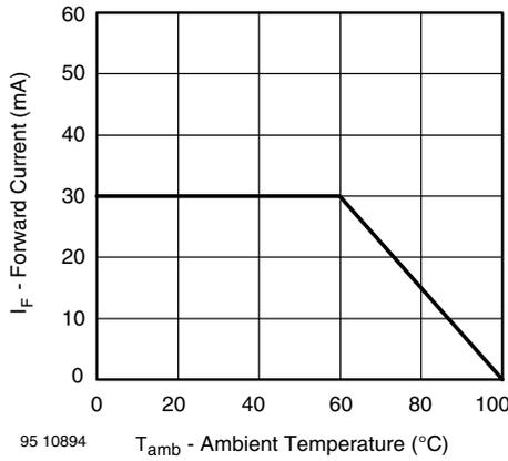
Fig. 1 - Forward Current vs. Ambient Temperature for InGaN
