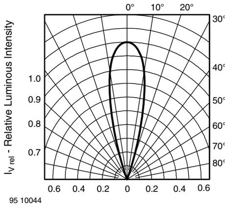
Fig. 2 - Relative Luminous Intensity vs. Angular Displacement
