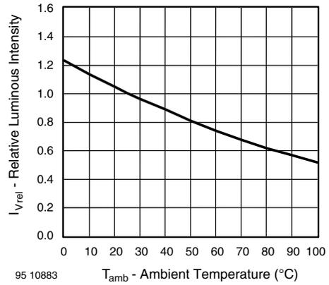
Fig. 4 - Relative Luminous Intensity vs. Ambient Temperature
