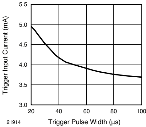
Fig. 11 - Trigger Current vs. Trigger Pulse Width
