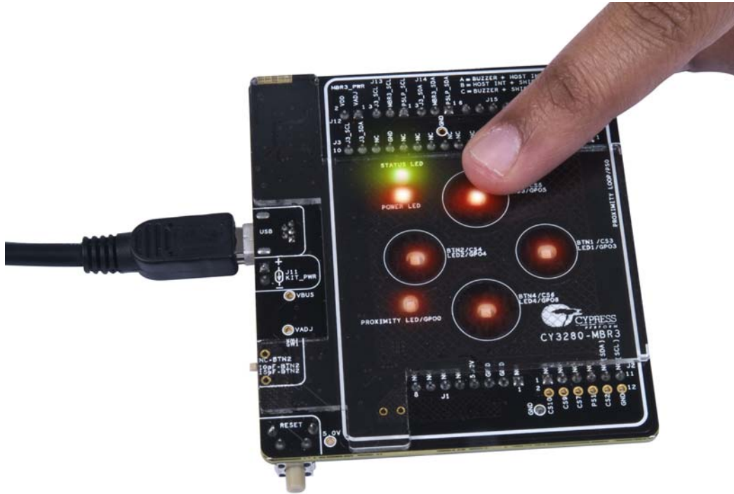
Figure 5-8. LEDs with 93 Percent Brightness on Button Touch
