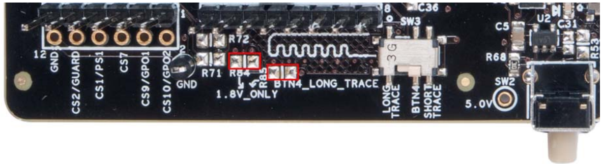
Figure 4-5. R84 and R85 for 1.8-V Operation
