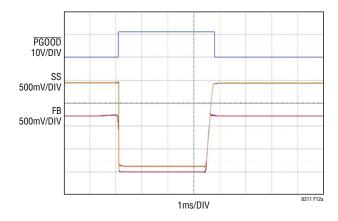
(a) Output Overshoot Control with  $C_{SS}$  = 1nF. LT8311  $V_{IN}$  Powered from a 12V Housekeeping Supply, Which Also Pulls Up on the  $\overline{PGOOD}$  Pin Through a 100k External Resistor
