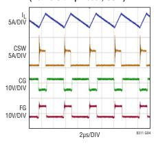
**Preactive Scheme Waveforms** (Active Clamp Reset, Light DCM)
