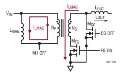
Figure 3. With FG On,  $I_{LMAG}$  Is Conducted Through  $M_{FG}$  to Ground on the Secondary Side When M1 Turns Off
