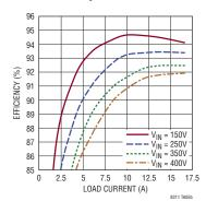
150V to 400V, 12V/16.7A, 200W No-Opto, Active Clamp Isolated Forward Converter
