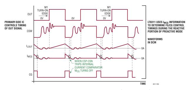
Figure 6. During the Reactive Portion of Preactive Mode, the LT8311 Turns Off  $M_{CG}$  When the Current in  $M_{CG}$ ,  $I_{MCG}$ , Trips the LT8311's Internal Current Comparator. The Inputs to the Comparator Are CSP and CSN and the Current Sense Trip Voltage Is Programmed by Choosing Appropriate CSP/CSN Series Resistors
