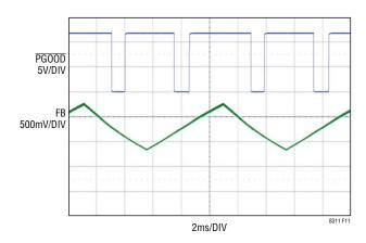
Figure 11. Power Good Activates ( $\overline{PGOOD}$  = Low) When the LT8311's FB Pin Voltage Is Within ±7% of Its Regulated Target (1.227V). The  $\overline{PGOOD}$  Pin Is Pulled Up Externally to a 12V Housekeeping Supply Through a 100k External Resistor
