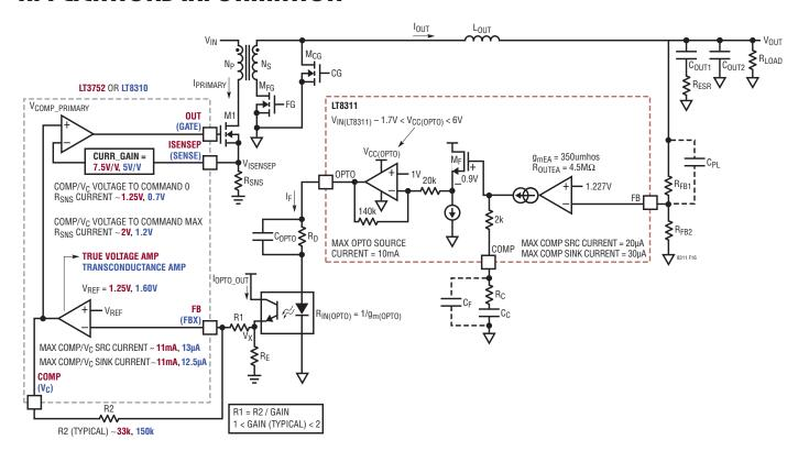
Figure 16. Forward Converter Voltage Feedback Loop with LT8311 on Secondary Side and LT3752 (or) LT8310 on Primary Side
