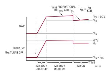
Figure 4. Detail of Region 3 from the Timing Diagram in Figure 2. When  $M_{FG}$  Turns Off in Active Clamp Reset,  $I_{LMAG}$  Initially Slews Up SWP's Voltage from  $V_{IN}$  to  $V_{CL}$  + 0.7V, at Which Point M2's Body Diode Turns On and Allows  $I_{LMAG}$  to Flow into  $C_{CL}$
