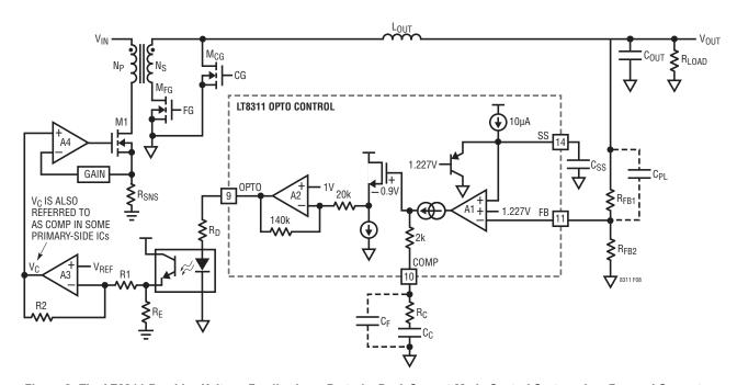
Figure 8. The LT8311 Provides Voltage Feedback, as Part of a Peak Current Mode Control System, in a Forward Converter
