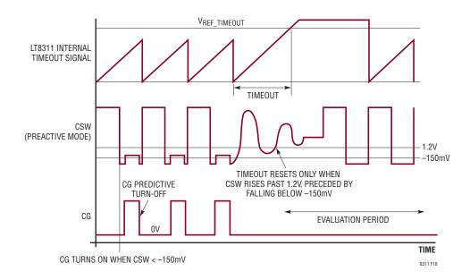
Figure 18. If Timeout Is Triggered in Preactive Mode, LT8311 Shuts Down All Synchronous Conduction and Starts the Evaluation Period (Note: CSW's ringing waveform is caused by the inductor current getting to OA.)
