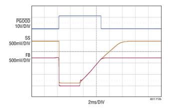
(b) Output Overshoot Control with  $C_{SS}$  = 33nF. LT8311  $V_{IN}$  Powered from a 12V Housekeeping Supply, Which Also Pulls Up on the  $\overline{PGOOD}$  Pin Through a 100k External Resistor
