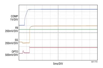
Figure 10. Opto Control Operation at Start-Up
