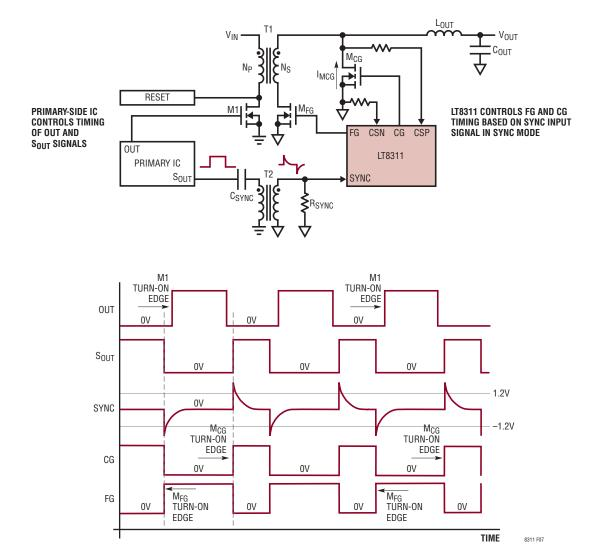
Figure 7. In SYNC Mode, the Primary Side IC Sends  $S_{OUT}$  Signals Through a Pulse Transformer to the LT8311's SYNC Pin. SYNC < 1.2V Turns on  $M_{FG}$  and Turns Off  $M_{CG}$ . SYNC > 1.2V Turns On  $M_{CG}$  and Turns Off  $M_{FG}$
