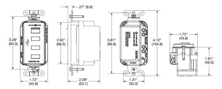
Note: For use with boxes deeper than 1.5" with internal AC/MC clamps.
