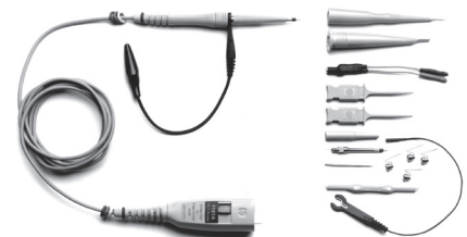
1165A 500 MHz passive probe
