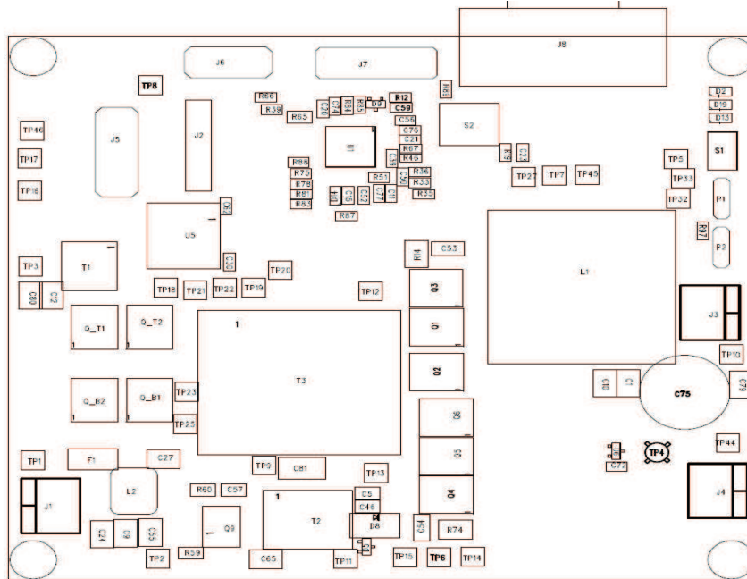
Figure 15. UCD3138HSFBEVM-029 Top Layer Assembly Drawing (top view)
