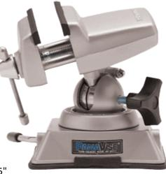
• Nylon jaws offer excellent electrical insulation and gentle holding power [continuous heat tolerance up to 200°F (93°C), intermittent heat to 300°F (149°C)]. Interchangeable jaws available
