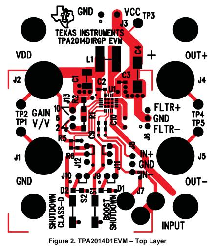
**Note:** C4 has two separate pad sizes. One is for a 1210 ceramic capacitor, and the other is for a size "C" tantalum capacitor. Do not populate more than one at a time.
