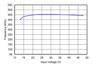
Figure 3. Frequency vs Input Voltage (I<sub>OUT</sub> = 100 mA)
