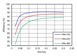
Figure 2. Efficiency vs Load Current
