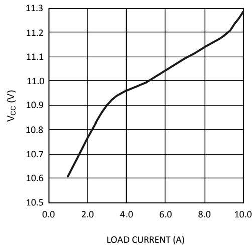
**Figure 5. V<sub>CC</sub> Voltage vs Load Current**
