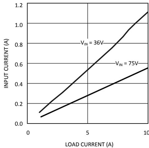
**Figure 2. Input Current vs Load Current and  $V_{IN}$**
