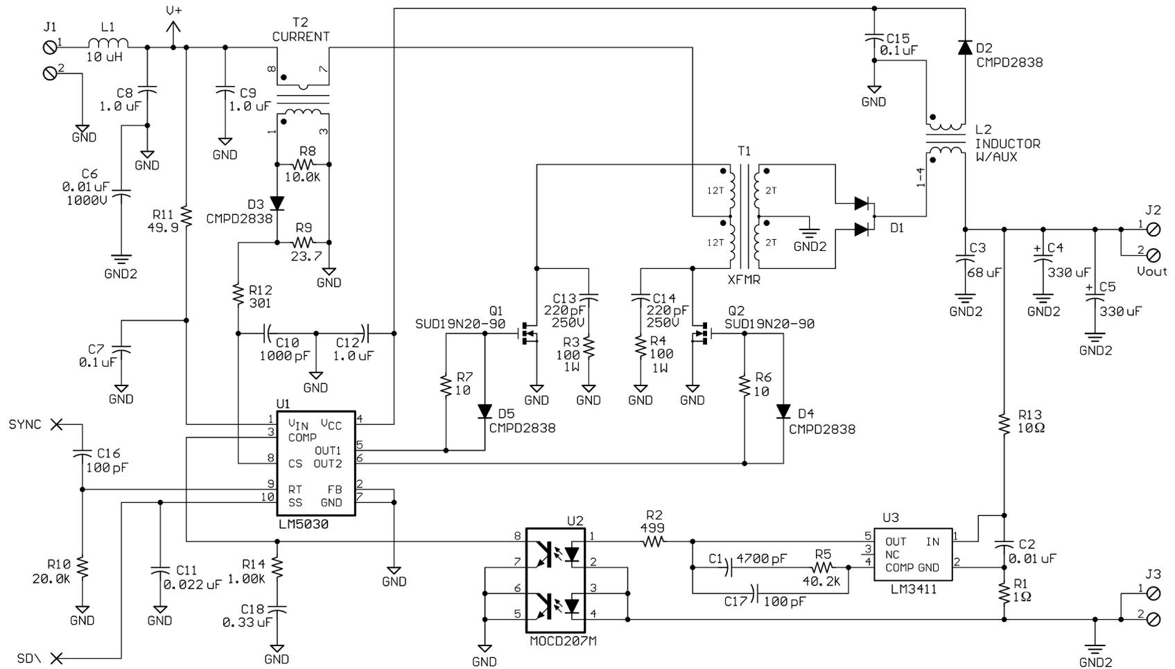
Figure 10. Board Schematic
