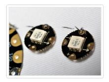
Start by stitching the ground bus from GND on Flora to the (-) pads on each pixel.
