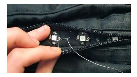
Then connect up the short data connections between each pixel. Be sure to seal the knots with clear nail polish or Fray Check.
