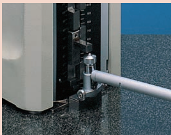
Bore gage zero-setting
