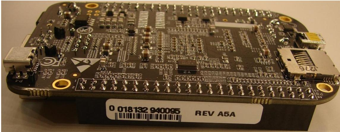
**Figure 78. Third Phase Serial Number and Revision Location**
