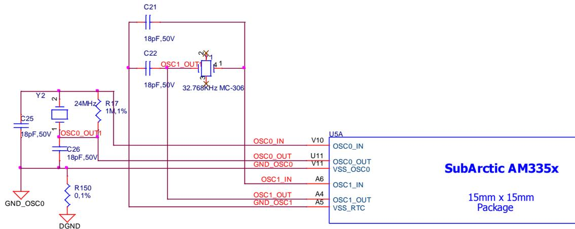
Figure 30. Processor Crystals
