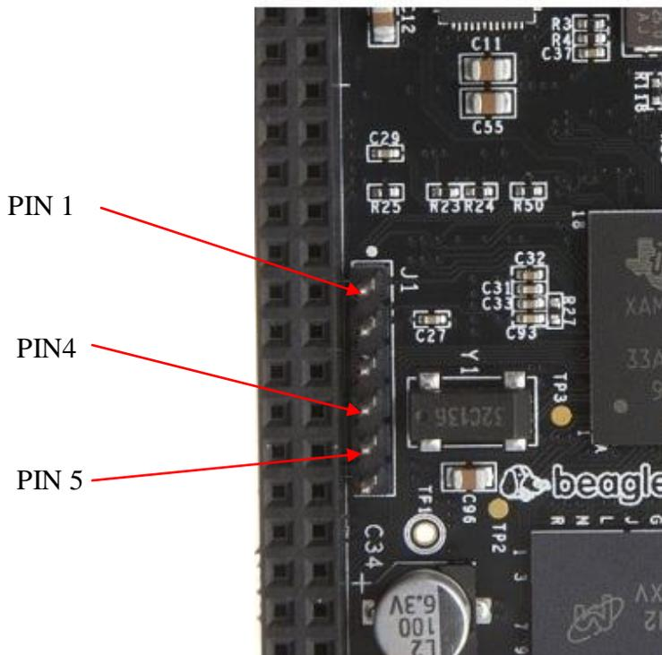
**Figure 56. Serial Header**
