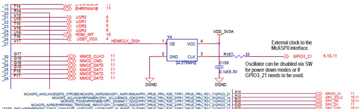
Figure 45. 24.576MHZ Oscillator
