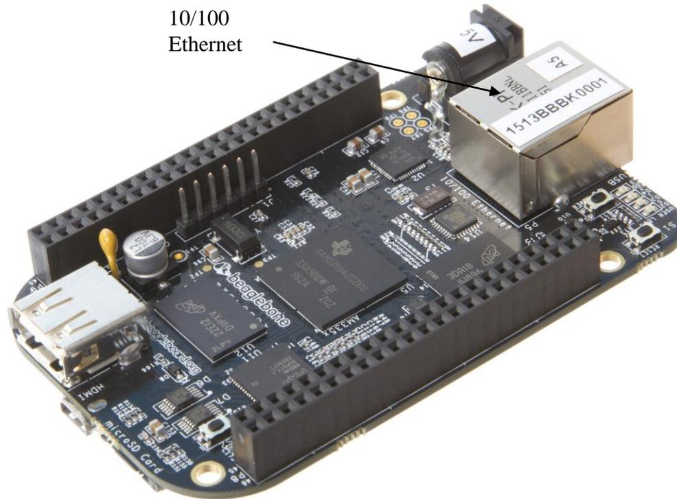
**Figure 60. Ethernet Connector**
