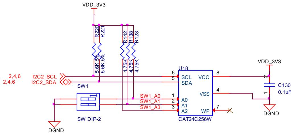
**Figure 61. Expansion Board EEPROM Without Write Protect**
