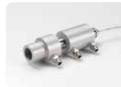
The air/water cooled housing allows the sensor to withstand ambient temperatures which exceed the normal 70°C limit. Air or water (depending on the degree of cooling required) flows into one of the fittings on the side and out of the other. To prevent condensation forming on the lens, the air/water cooled housing is supplied complete with an air purge collar. Please note, the air/water cooled housing must be ordered with the sensor and cannot be fitted by the user.
