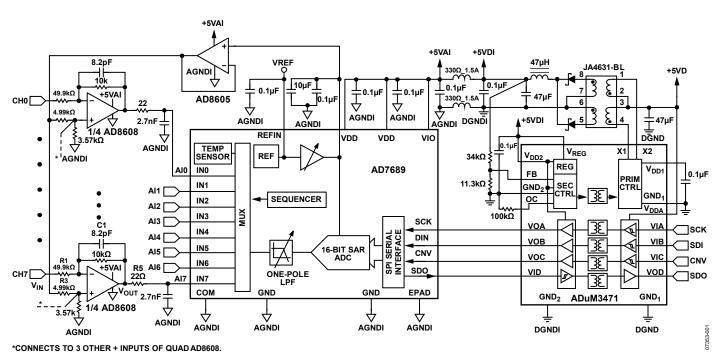
Figure 1.16-Bit, 250 kSPS, 8-Channel Data Acquisition System (Simplified Schematic: All Connections and Decoupling Not Shown)
