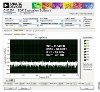
Figure 5. FFT with a Kaiser Window (Parameter = 20), 20 kHz Input, 250 kSPS Sampling Rate
