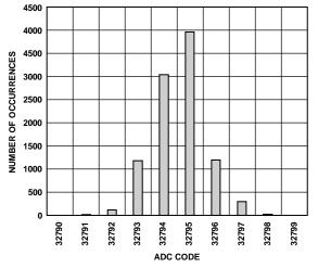
Figure 4. DC Histogram for a 0 V Input, 10,000 Samples
