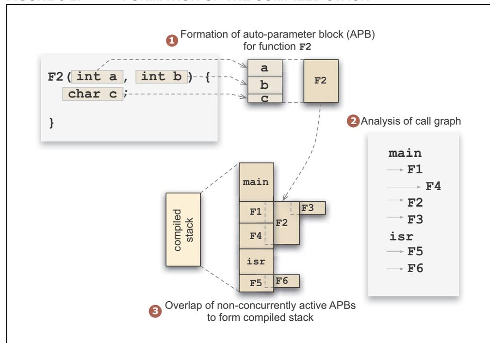
Each function in the program is allocated a block of memory for its parameter, `auto` and temporary variables. Each block is referred to as an auto-parameter block (APB). The figure shows the APB being formed for function `F2()`, which has two parameters, `a` and `b`, and one `auto` variable, `c`.
