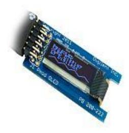
The Digilent PmodOLED Peripheral Module is perfect for embedded applications requiring small, complex visual output. It is compatible with Digilent's PIC32-based Cerebot development boards (TDGL008, TDGL009, TDGL010), and can be easily connected to any system using standard IDC connectors and cables. An SPI interface is used to communicate with module.
