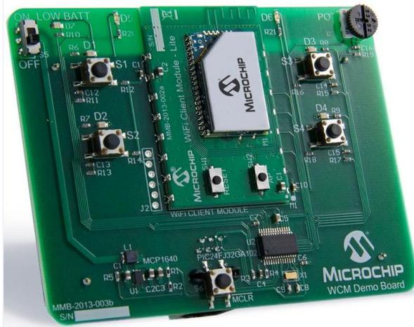
The Microchip WiFi Client Module Development Kit 1 is designed to enable the user to quickly and easily connect to a cloud based server such as Amazon AWS. The kit includes the WCM demo board utilizing a Microchip WiFi Module MRF24WG0MA and an application microcontroller PIC32. The device allows commissioning to router and then connects to an Amazon AWS server. The AWS account and AMI must be established prior to module commissioning. Microchip offers a free AMI image on Amazon AWS.
