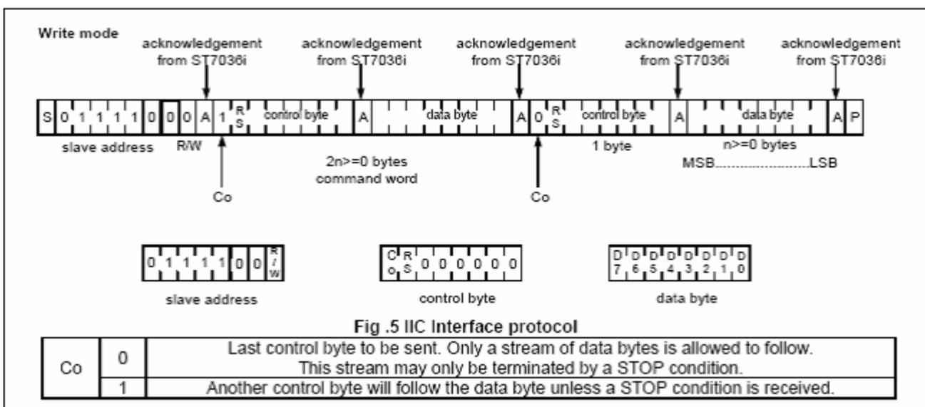
During write operation, two 8-bit registers are used. One is data register (DR), the other is instruction register(IR).
