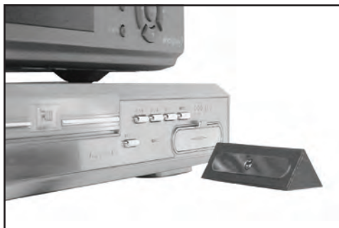
Example 2: Mount the IR Emitter horizontally using the supplied sticky pad. Ensure the LED is facing the IR sensor on your source equipment.
