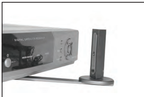
Example 1: Mount the IR Emitter vertically using accessories 1 and 2. Ensure the LED is facing the IR sensor on your source equipment.
