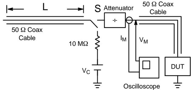
Figure 7. Simplified Schematic of a Typical TLP System
