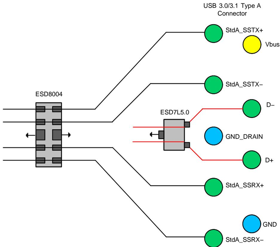
Figure 14. USB 3.0/3.1 Layout Diagram
