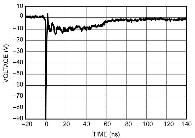
**Figure 2. IEC61000-4-2 -8 kV Contact ESD Clamping Voltage**
