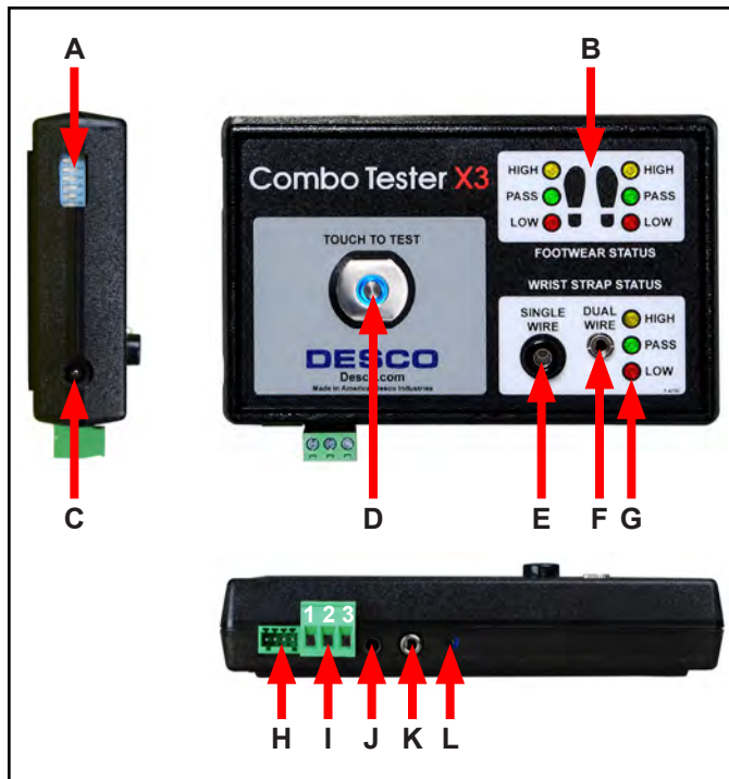
Figure 2. Desco Combo Tester X3 features and components
