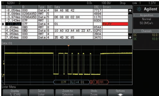
Figure 1: Hardware-based decoding quickly reveals serial communication errors.
