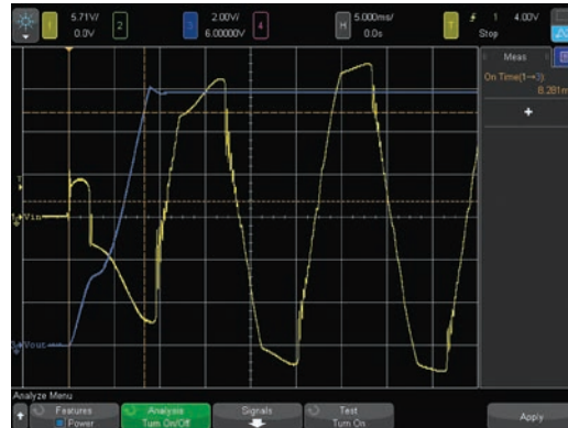
Figure 8 The turn-on analysis measures the time taken to get to the steady output voltage of the power supply after the input voltage is applied.
