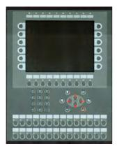
The Terminal E900 VT has 28 external function keys supported by the built-in expansion card IFC 64E. The expansion card is selected automatically in expansion slot 1 when you select the terminal E900 VT under **File/Project Settings**.
