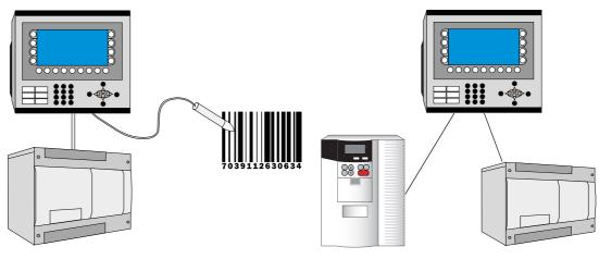
Operator termial with contro system and barcode reader connected
