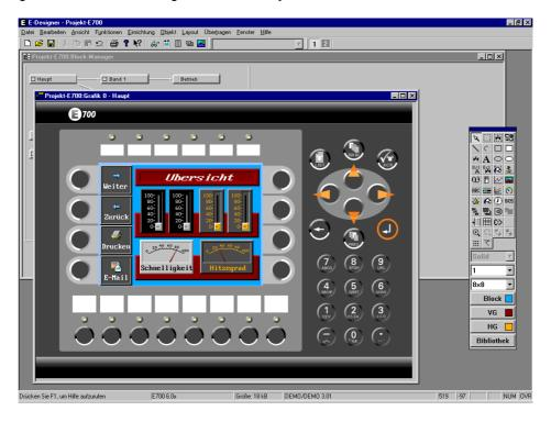
The terminal is to a large extent object oriented, i.e. first an object is selected and then the function the object is to have. All types of signals are defined on this principle.
