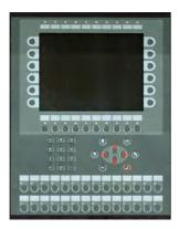
The Terminal E900 VT has 28 external LEDs supported by the built-in expansion card IFC 64E. The expansion card is selected automatically in expansion slot 1 when you select the terminal E900 VT under **File/Project Settings**.
