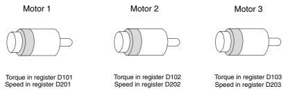
Register D0 is defined under **Setup/Index register** as Index register 1. The value in the register will determine for which motor the torque and speed are to be shown.
