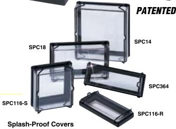
Splash-proof covers provide additional protection for instruments. Following NEMA 4 (IP66) guidelines for windblown dust and rain, splashing water and hose-directed water, SPC covers form a protective seal around the instrument bezel. Available in 1/4, 1/8, 1/16 and % DIN sizes for compatibility with most panel meters.
