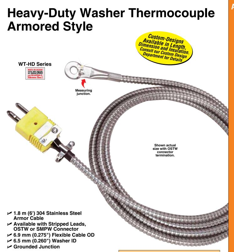
Rugged thermocouple, for surface mount applications, has a washer mounting surface and an overall dimension of 17.3 mm (0.680") OD, with a 6.6 mm (0.260") mounting hole of 304 SS material. Attached to the mounting surface: 1.8 m (6') of 304 SS flexible armor cable with stripped wire ends. Armor cable has 6.9 mm (0.275") OD, with 1.78 mm (0.070") washer thickness. Standard male connectors are available for cold-end termination. Rated to 480°C (900°F) for Type K only.
