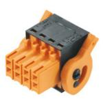
Female connector with integral cross-connection and clear printing for uninterrupted relaying of potential at full current-carrying capacity with the maximum cable crosssection. The cross-connection is positioned vertically between the poles of rows directly on top of each other. Conductor connection with tension clamp system with straight outlet and 3.5 mm pitch. Flange and release lever available. Packed in cardboard box.
