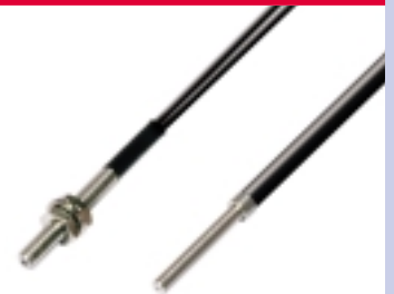
E32-C31 (Diffuse, M3 threaded 75 mm range) E32-C41 (Diffuse, M3 threaded 35 mm range) E32-C42 (Diffuse, 2 mm dia., 6 receivers)
