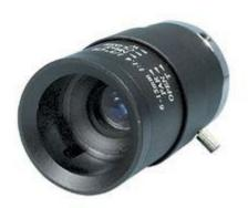
Take the guess work out of your CCTV installation. Defender Security offers a wide range of options to make your job easier. Vari-focal lenses feature fully adjustable focal lengths reducing the lenses you need to stock. All lenses are CS mount and are ideal for 1/3" image format CCDs. They are available in manual, DC and video auto-iris. The recommended minimum object distance is greater than 8".
